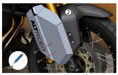
Start by putting thread locker on the last few threads of the (2) M6 x 35 fasteners and then assemble the guard as shown in the exploded view above. (2) spacers, guard, (2) M6 finishing washers, (2) M6 x 23 flat head fasteners. Use a 4mm allen tool to tighten the fasteners.
