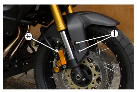
Use a 4mm allen tool to remove the (2) OEM fasteners. Repeat for the other side of the fender.
